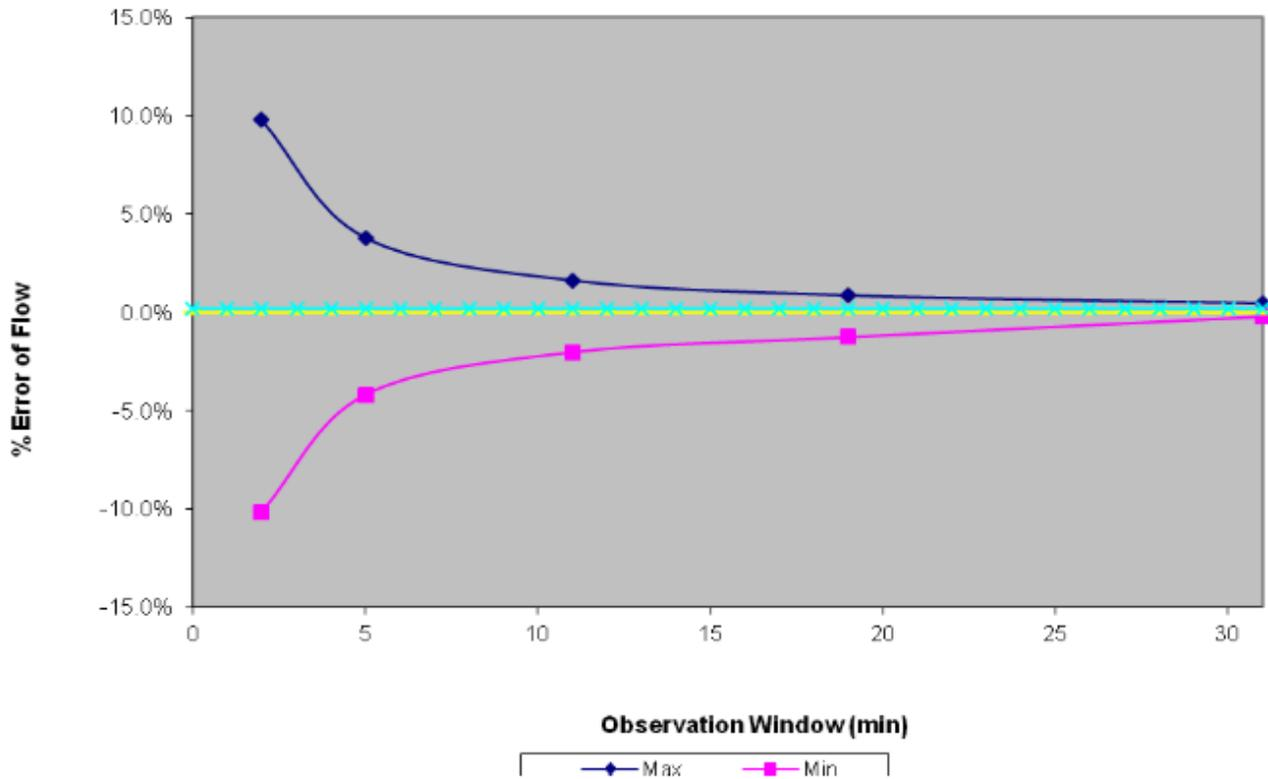
Table 13: The graph below shows the trumpet curve during the last two hours of testing at 600 mL/Hr. This graph shows the average percentage error, maximum percentage error, and minimum percentage error curves. The test was performed according to the IEC 60601-2-24 Standard.
